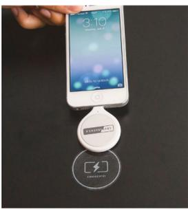
Perfect for boardrooms, workstations, and common spaces, ChargeSpot is conveniently installed beneath table surfaces to create a wireless charging spot while maintaining the structural and aesthetic integrity of the furniture. In addition, wireless charging through magnetic induction has proven to be extremely effective, charging devices at 90% the speed of a typical charging cable.
